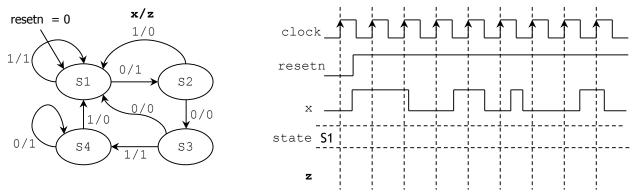
Provide the state diagram (in ASM form) and complete the timing diagram of the FSM whose VHDL description is listed below. (15 pts)
